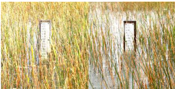
Left: A staff gauge shows water level in relation to something else. This one just north of Main Park Road, in the heart of Taylor Slough, read 5.18 feet above sea level on October 10, 2020—the date of my original foray into the flooded park. Just 14 days later, it read 5.66 feet. Almost half a foot increase may seem tiny, but the pictures show just how much less “grass” emerges from the River of Grass with that huge-for-the-Everglades increase. NPS Photos by Michelle Collier.
