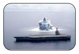
The first of what will be several tests, aims to demonstrate the ship's ability to withstand a shockwave. There will be several "Full Ship Shock Trials (FSSTs) in the coming months off the coast of Florida. The USS Gerald R Ford is the "the newest and most advanced aircraft carrier" in the Navy, and can be deployed once it has passed the series of action-ready tests.
